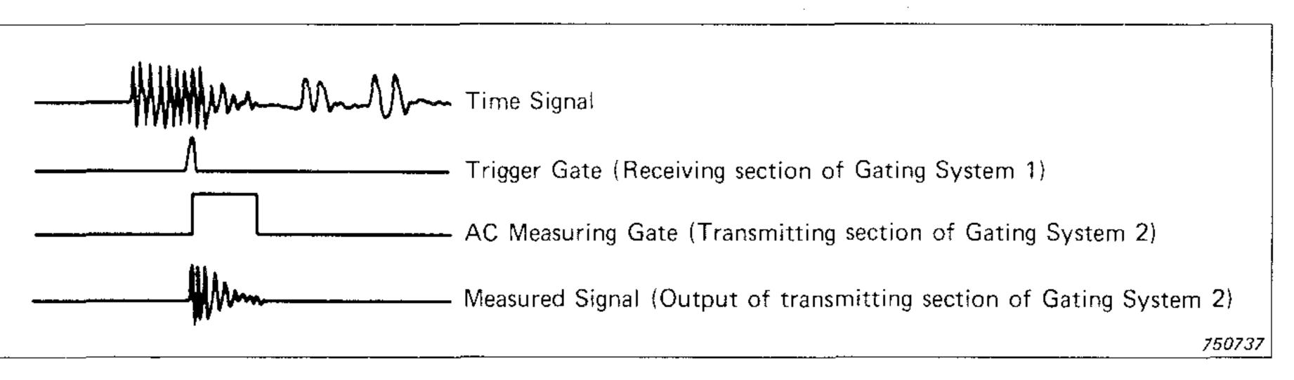
Fig.16. Setting of gates to measure the various reflections with the set-up in Fig.15.
