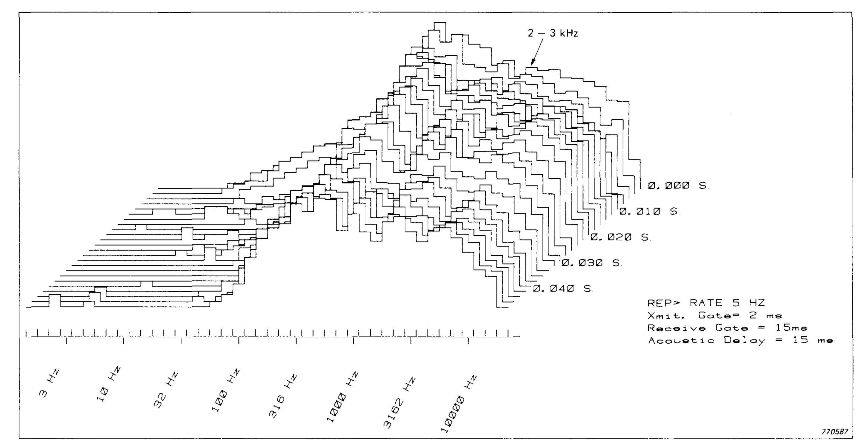
Fig.19. 3 D plot of lecture room showing how the frequency spectra change with time. 0—50 ms time axis. Receiving gate 15 ms Notice the "Flutter Echo" at 2 kHz
