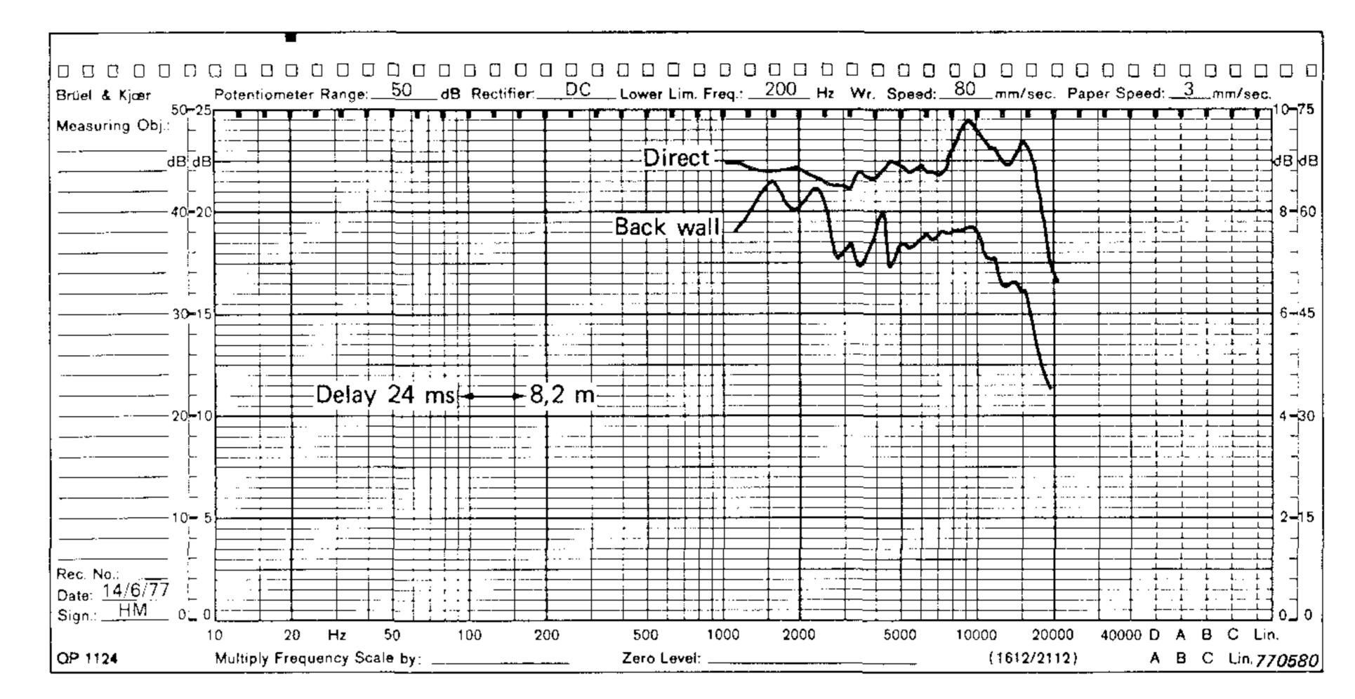
Fig.14. The reflected sound from the back wall relative to the direct sound from the loudspeaker
