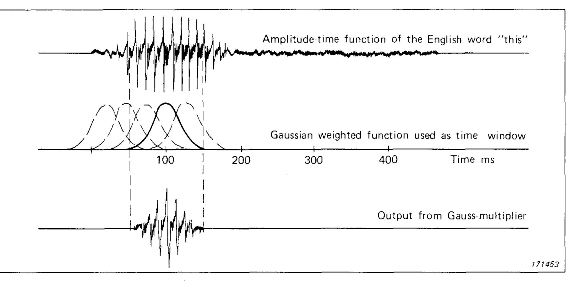
Fig.27. The operation of the Gauss Impulse Multiplier 5623
