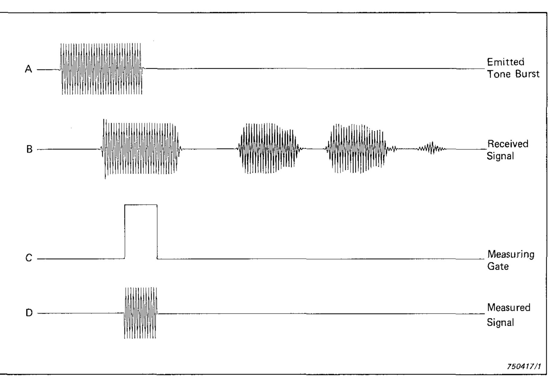
a selective measurement in the time domain just as frequency analysis is a selective measurement in the frequency domain. A tone burst is transmitted from a loudspeaker and measured at the listening position as indicated in Fig.1.
