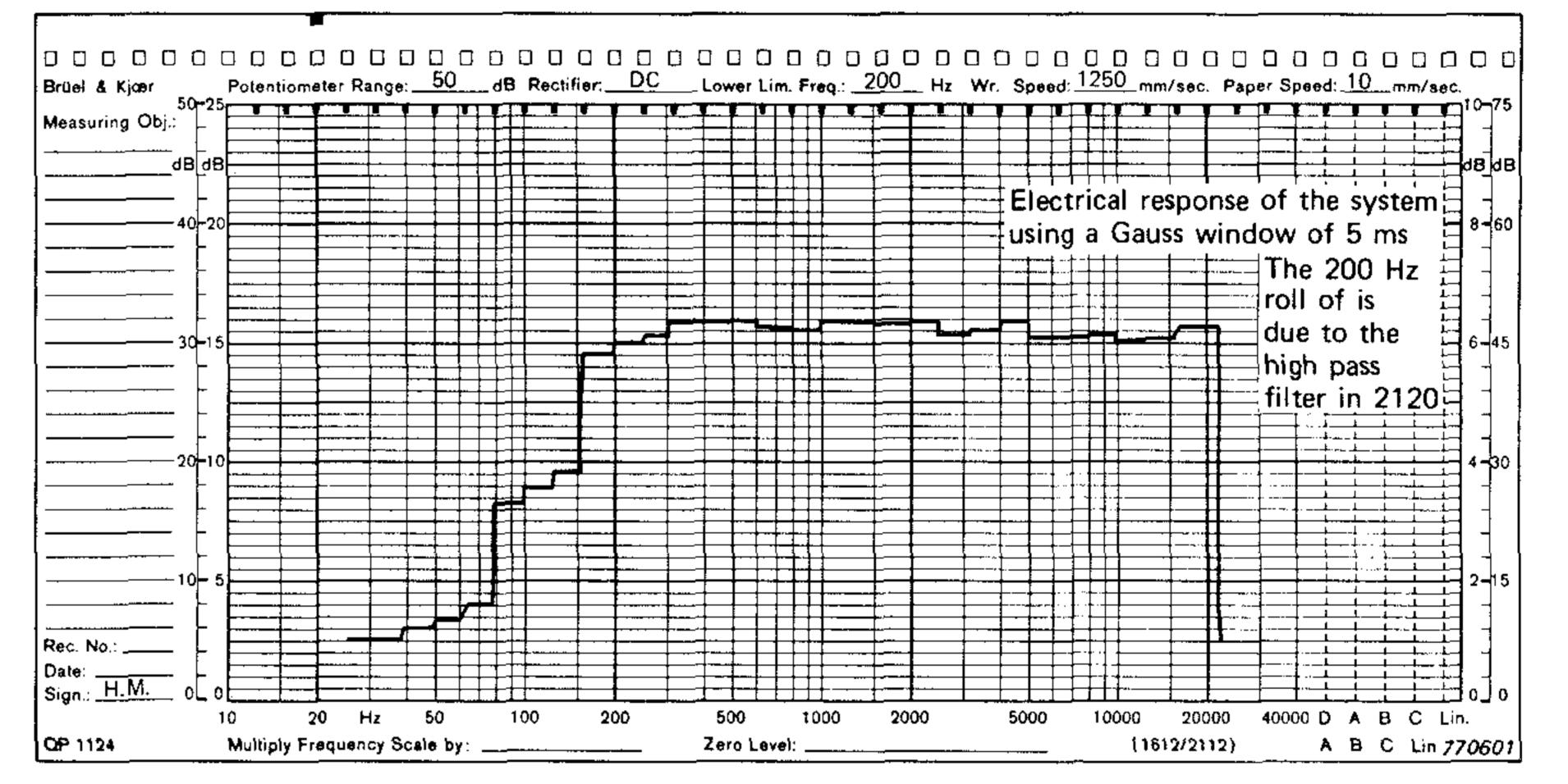
Fig.26 shows the electrical response of the system using the Gauss Impulse Multiplier 5623. The 200 Hz roll off is due to the high pass filter in 2120.
