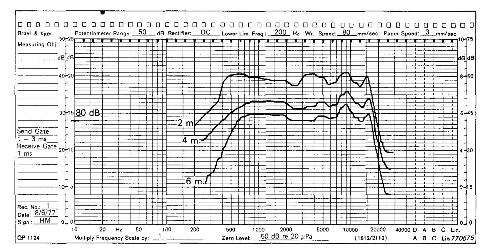
Fig.8. "Free-field" measurements of the loudspeaker used
