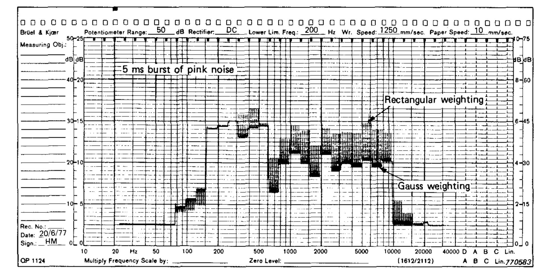
should be used — if any. This is described in detail in Bob Randall's Application Note (Ref.10). However using the 1/3 octave resolution the influence of the weighting function is almost negligible as can be seen from Figs.25 and 26.
