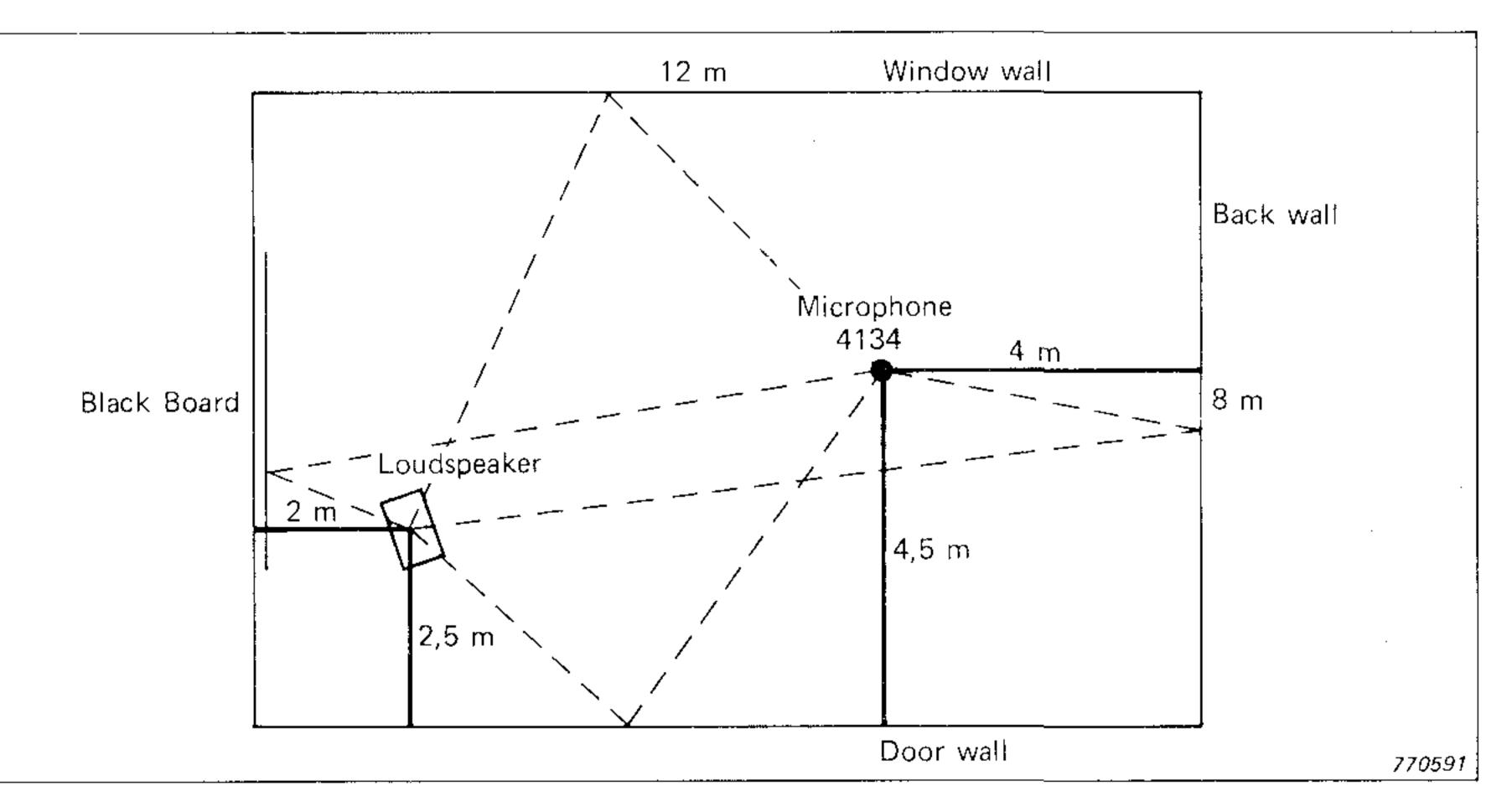
Fig.7. Schematic drawing of the lecture room
