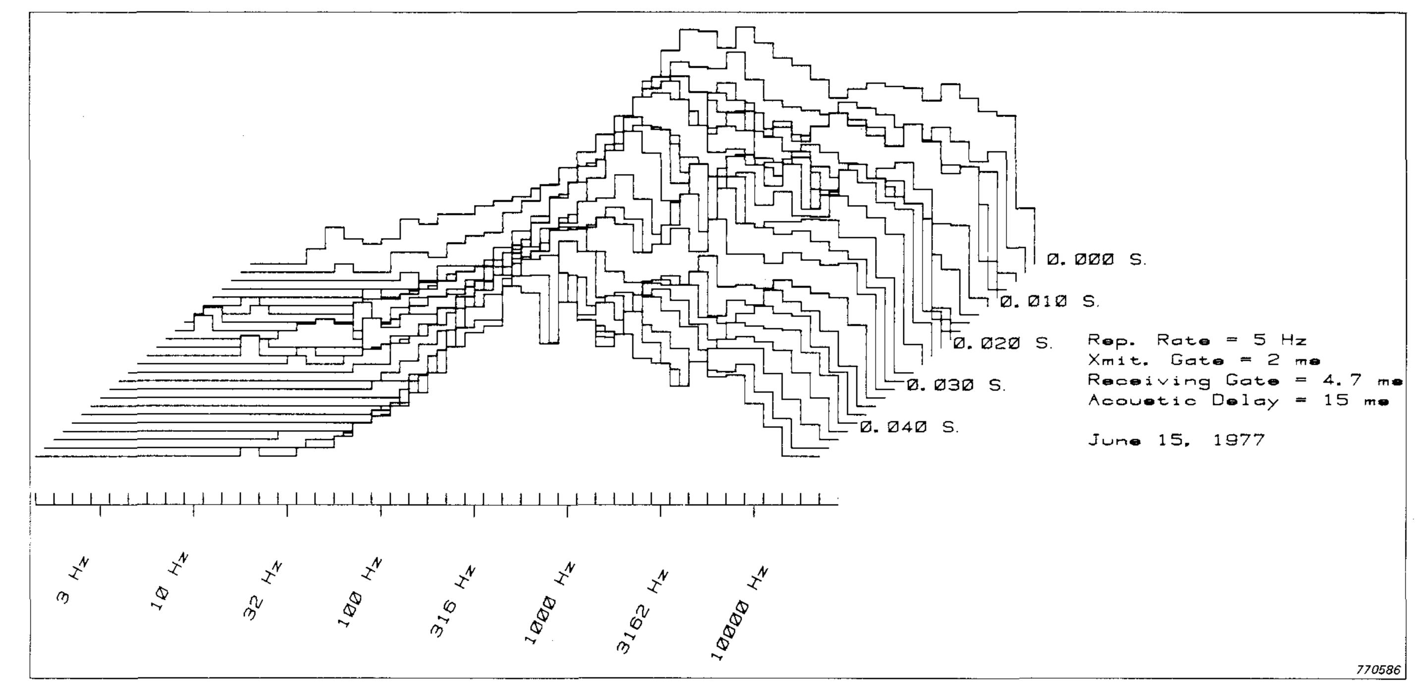
Fig.18. 3 D plot of lecture room showing how the frequency spectra change with time. 0-50 ms time axis. Receiving gate 4,7 ms
