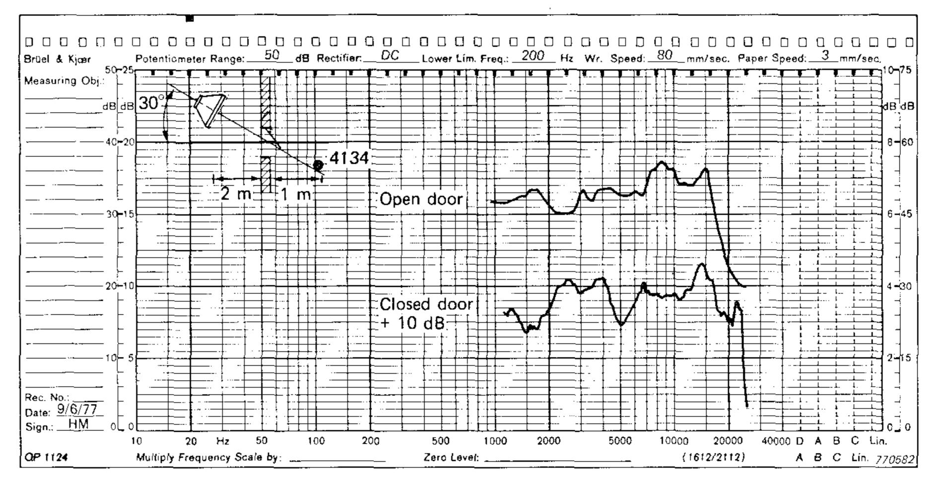
door "on axis" has the lowest attenuation in the critical range 3 kHz. Here it is only 18 dB.
