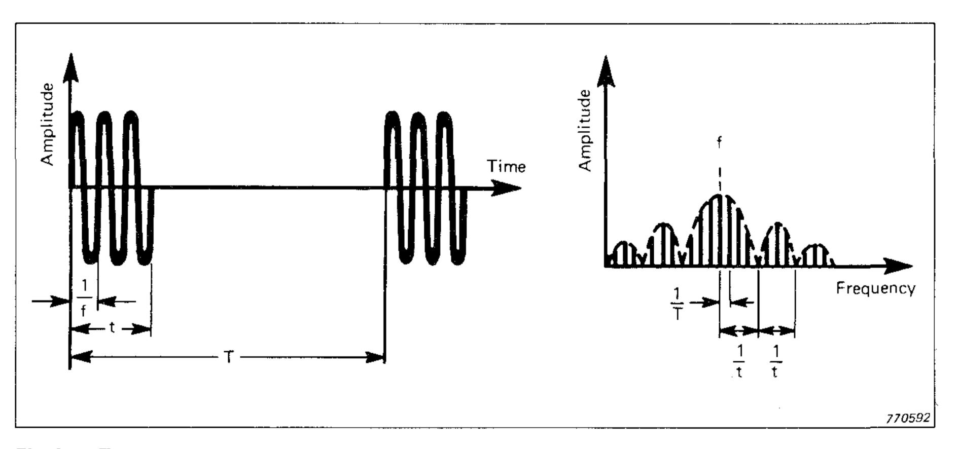
Fig.4. Time and frequency spectra of gated sine wave. Notice that a narrow time spectrum corresponds to a broad frequency spectrum and vice versa
