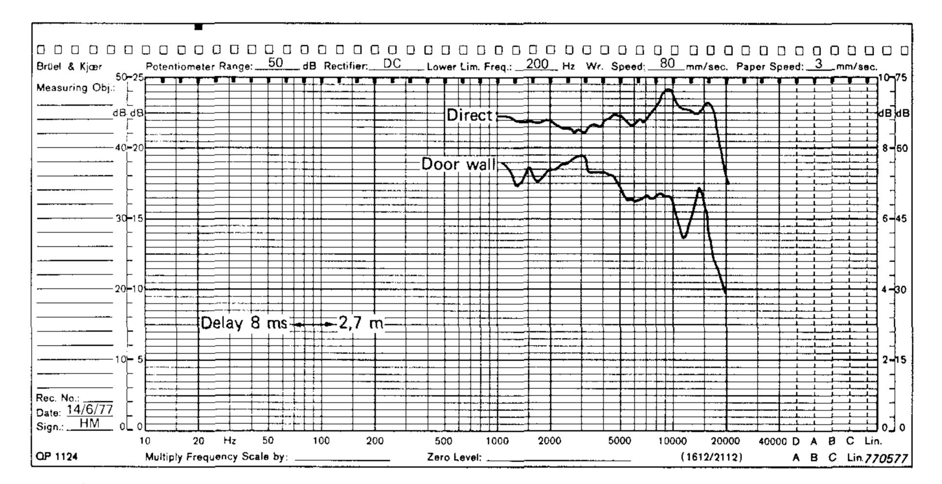
First of all, it is seen that most of the reflections on average are about 10 dB down, but they do not die down at the same rate at all frequencies. Since the four curves are different, they also indicate that the decay rates at the various frequencies are different in the different directions.
