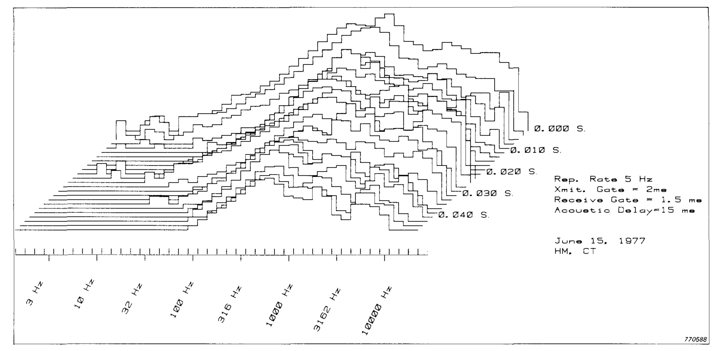
Fig.17. 3 D plot of lecture room showing how the frequency spectra change with time. 0-50 ms time axis. Receiving gate 1,5 ms
